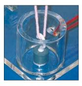
This Tension Hook is to be used in the small fixed cylinder.
