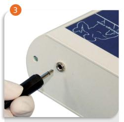
Ensure the lead running from the syringe is plugged into the circular socket at the back of the Feedback Console
