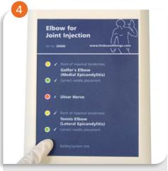
Press the 'Battery/system test' button at the bottom of the front panel of the Feedback Console. All the lights should illuminate
